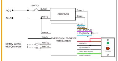
1.DO NOT MATE CONNECTOR UNTIL INSTALLATION IS COMPLETE AND AC POWER IS SUPPLIED.
