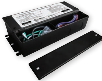
Power Supply for 24V Strip Light Input: 120V-277V AC Output: 24V DC Power: 60W~300W
